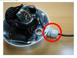
5. Pass the camera end of the power/video cable through side conduit hole. Using wrench or pliers, carefully tighten the weather tight bushing into the side conduit hole.
